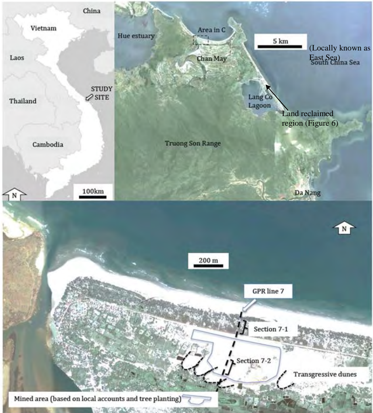
Figure 1. Study site in Chan May embayment, approximately 35 km north-northwest of Danang, central Vietnam. A GPR profile (Line07) was collected from modern shoreline to a transgressive dune across a sand-mined area. Section 7-1 and 7-2 shown are figure 2 and 3 respectively, distinguishing the difference between prograding beach radar facies and sand-mined radar facies.
