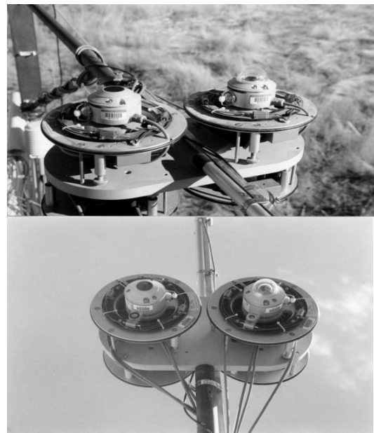
Figure 2- The upper picture shows the facing up pyrgeometer (left) and pyranometer (right). The lower picture shows the same instruments as in the middle picture, but facing down.
