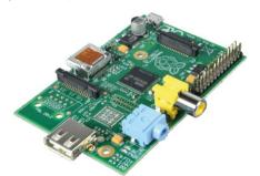
Figure 2.3 Raspberry Pi (Raspberry Pi, 2016)
